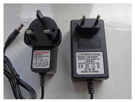
Here are two different charger types; however they both have an indicated output voltage of 8.4V which makes them suitable for charging 2 series Li Ion battery packs. However they differ in other ways. The one on the left has an output of 1 amp, so is fairly universal. A battery with multiple cell arrays will just take a fraction longer to charge. This example is not specifically marked as a Li Ion charger however, although it is. Both have charging (red) to Fully Charged (green) LED indicators.
