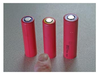
On the left are three different types of Lithium Ion battery cell. All are OEM (Original Equipment Manufacturer) and as such not intended for retail sale. Usually fitted with a protection board and rebranded, they will have a new outer wrapper with the retail brand on it. Left is the cell described, centre is another 18650 designed for high discharge, as such its capacity is lower at 2600mAh. On the right is a 207000, higher capacity and rated at 15 amps maximum safe discharge.
