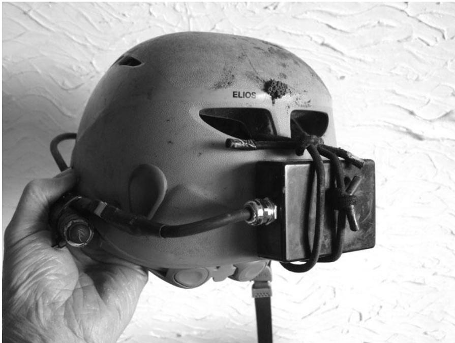
Above picture shows a battery pack securely mounted to a helmet. The beauty of this system is that it does not require the drilling of any extra holes.
