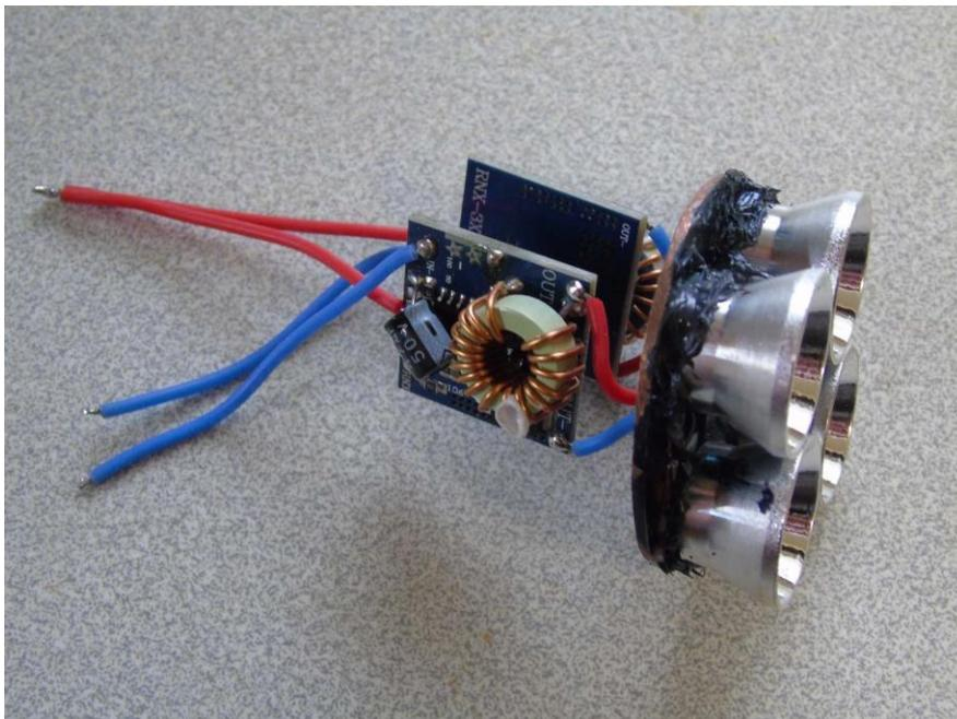
They have a control chip with no part number, seen this before, so was unable to get a data sheet. Evaluation therefore consisted of my lab tests which trashed a few. The ones left came in useful as they don't have mode memory so I was able to fit two, each to one pair of parallel emitters. So output of 3 amps gives 1.5 amps to each XHP 35.
