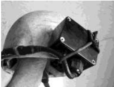
Above picture shows a battery pack securely mounted to a helmet in simple form. Use cable ties if required to secure the cable.
